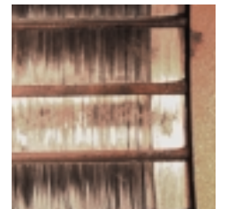
Microscopic examinations of the commutator surface provides information concerning the operational behaviour of the carbon brushes as well as regarding commutation
